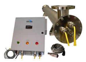
The electropolished, 316L schedule 10S stainless steel or CPVC UV Reactor houses more lamps per volume of flow than MP. This provides a more uniform UV intensity field and inherent degree of redundancy. Consider the scenario where a single lamp fails in a 2-lamp MP system versus an 8-lamp amalgam lamp system.
